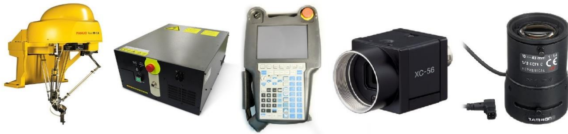
Figure 1. The robot, the control unit, the Teach Pendant, the camera and the objective [4], [5], [6]
